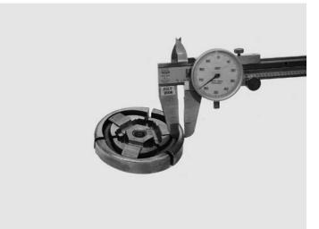
7.6 Inspect spring for cracks.
